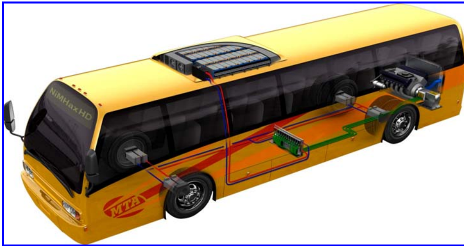
Fig 3. Early S.D. Metro bus with roof mounted NiMH batteries (1997)
